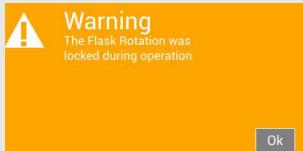
A process start is only possible when the rotational axis is unlocked and the warning message on the display is confirmed with [OK]!
