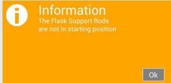
A process start is only possible when the support bars are in their respective end position and the warning message on the display has been confirmed with [OK]!
